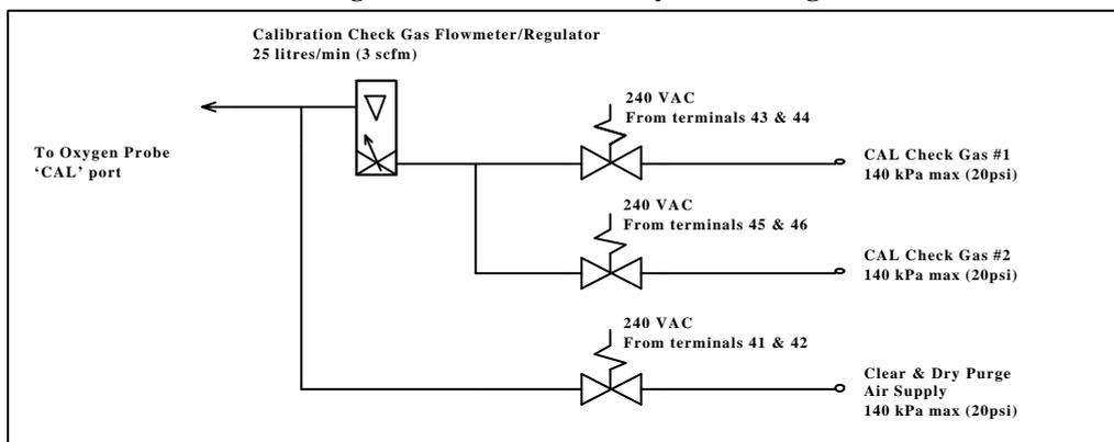
**Automatic Purge & Calibration check System Piping Schematic**
