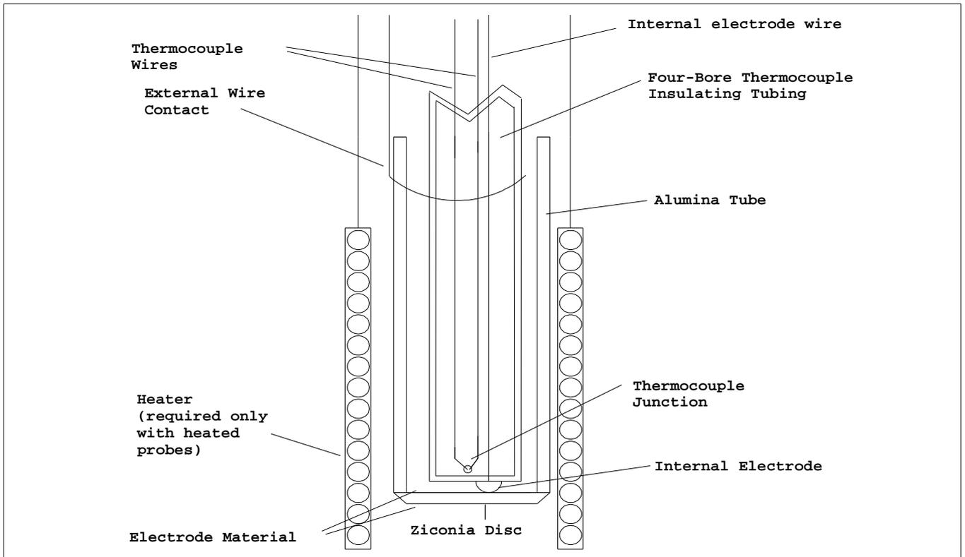
Schematic View of a Sensor Assembly
