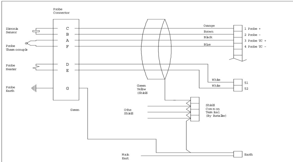
**Connection of Probe Cable for 1231 Model Heated Probes**
