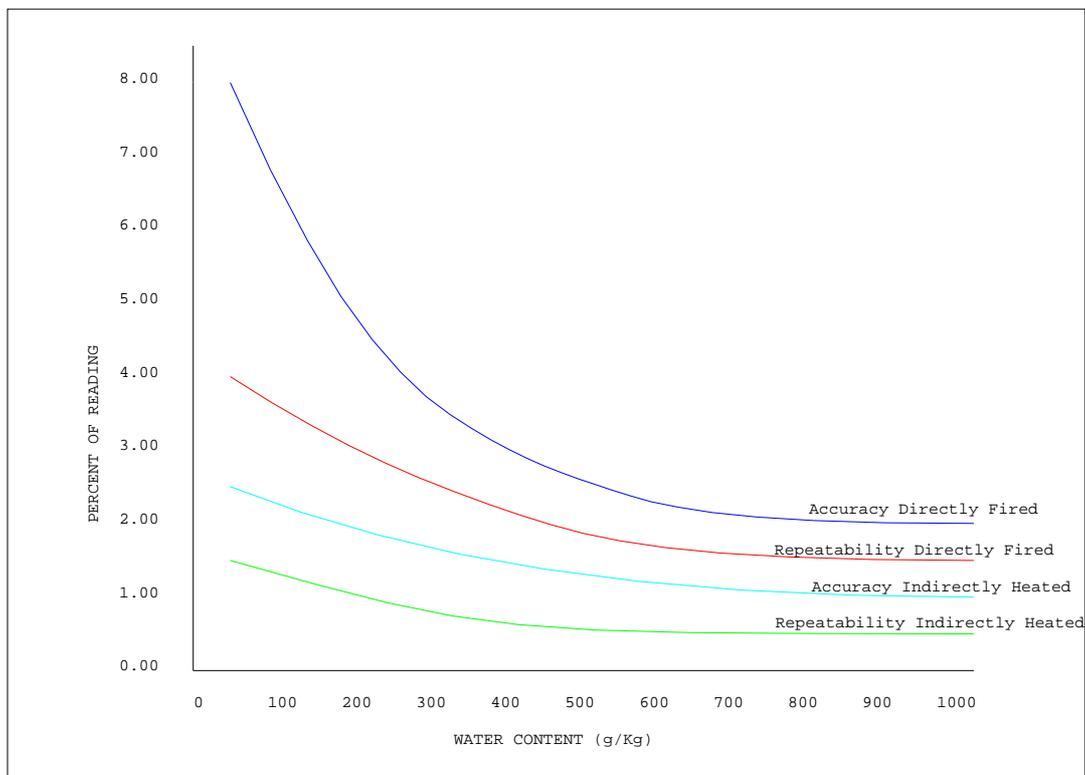
**Accuracy & Repeatability of 1635 Water Vapour % Analyser Readings**
