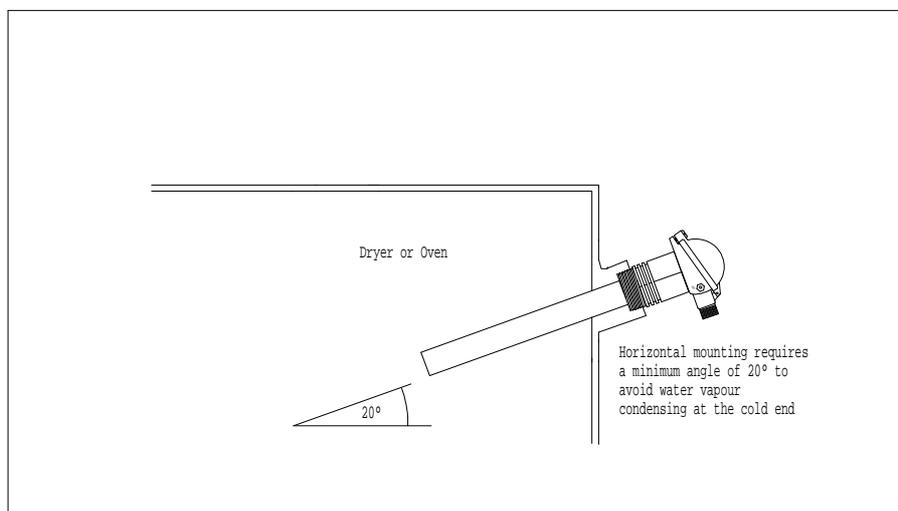
Installing an Oxygen Probe in the Dryer of Oven
