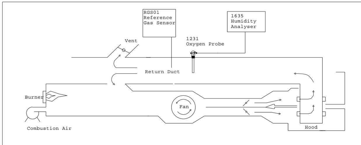
**Percent Water vapour Measurement in Directly Heated Dryer or Oven
