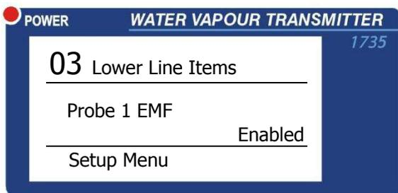
This function allows the operator to change the items that are available to be displayed on the lower line of the transmitter in Run Mode. If the word "Enabled" appears on the display for a selected lower line option, the measurement will be available to be shown on the display in the Run Mode by scrolling through the list using the DISPLAY  $\Delta$  and DISPLAY  $\nabla$  buttons.
