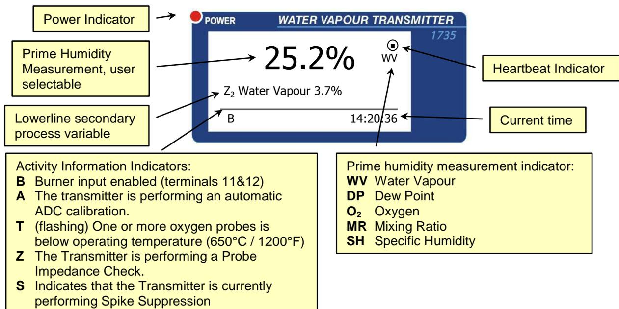
In Setup Menu the display is replaced with an interactive menu driven interface. While in the Setup Menu all other functions of the transmitter including reading inputs, calculation of process variables, checking of alarm conditions and retransmitting will continue to operate as normal.
