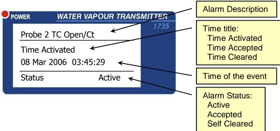
When a new alarm occurs, either a process alarm or an alarm that will appear in the common alarm list, the Alarm Light will flash quickly. The more new alarms there are, the faster the light will flash.
