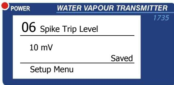
**Options:** 5mV to 100mV in 1mV increments
