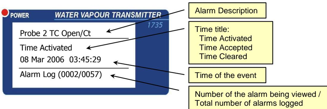
Use the OPTION  $\Delta$  and OPTION  $\nabla$  to scroll through the alarm events that have been saved in the alarm log. The alarm event will be transferred to the alarm log when the alarm has been cleared.
