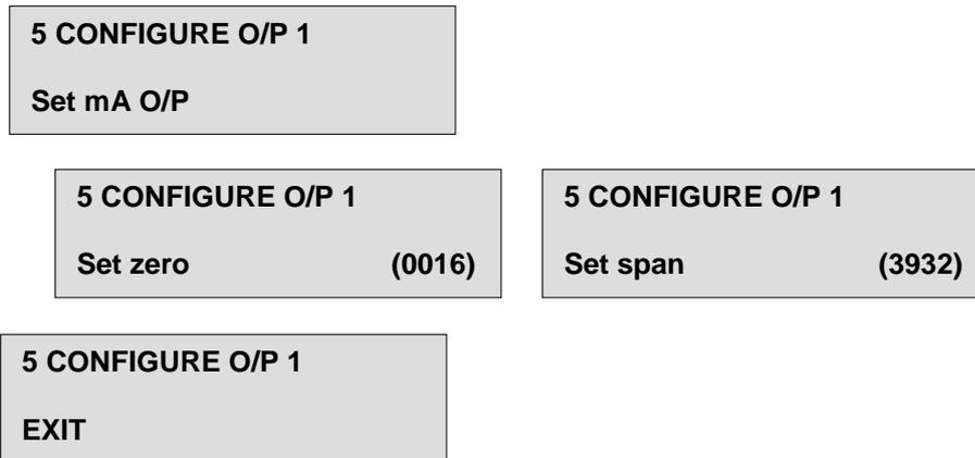
Repeat this output configuration process for Outputs 2 to 5.
