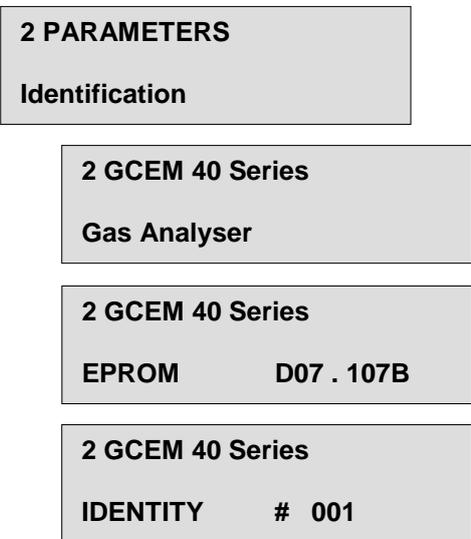
**Note:** The analyser identity number is set via the rotary switch on the processor card in the lid of the DDU.
