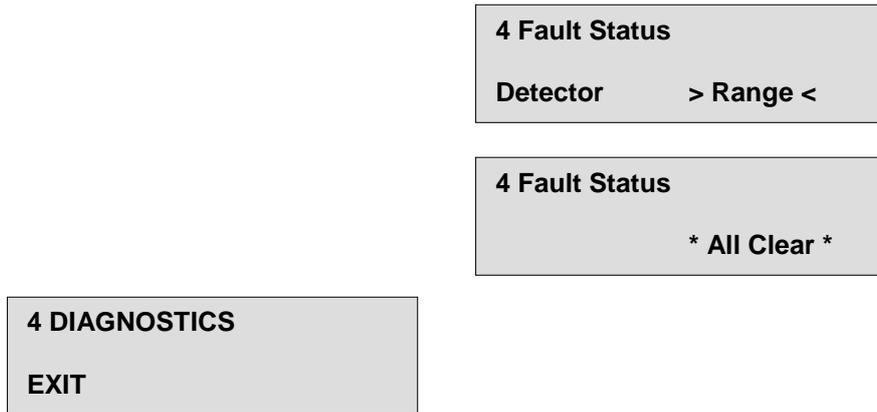
When no faults are detected the display will show the condition 'Fault Status' \* All Clear \*. The fault conditions which are tested for are as follows:
