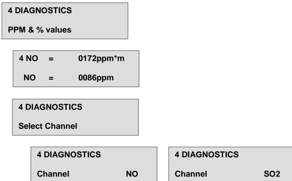
The analyser responds to the total number of molecules of gas within the measurement cell path and therefore measures the product of gas concentration multiplied by the optical pathlength. The basic measurement units for the analyser are therefore ppm x m or % x m. To obtain values in ppm (or %) this basic measurement must be divided by the measurement cell pathlength. Both ppm.m (or %.m) and ppm (or %) values are displayed.
