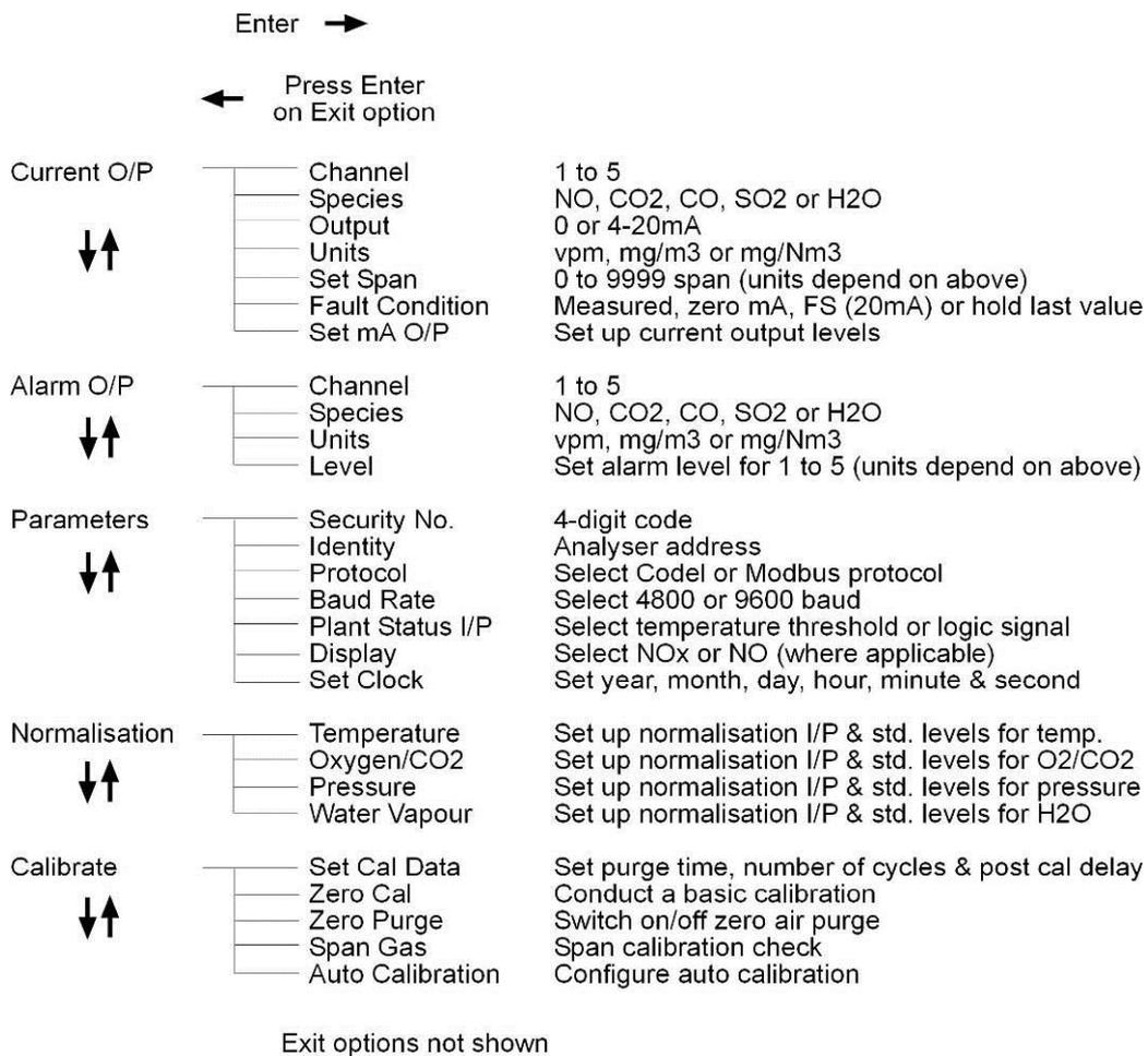
**Figure 4: Program Tree for the Set-Up Mode**
